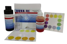
AQUA-XL Swimming Pool Test Kit is used to check the chlorine and pH level of swimming pool water. Regular testing ensures proper maintenance of chlorine & pH in swimming pool water.
